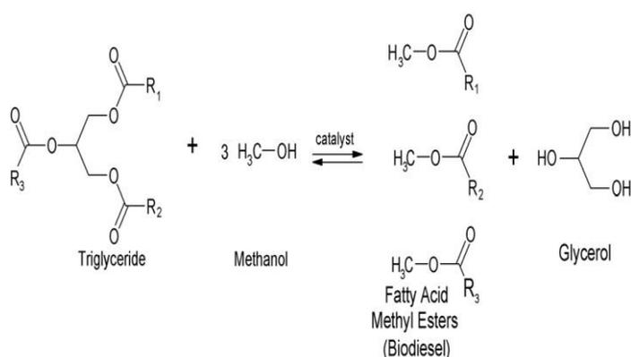
**Fig. Transesterification reaction of triglyceride and methanol to fatty acid methyl esters (biodiesel) and glycerol.**
