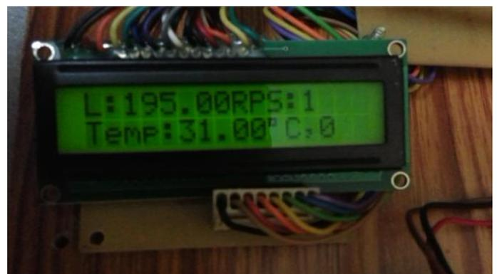
**Fig 3 LCD Display showing Level,RPS & Temperature**
