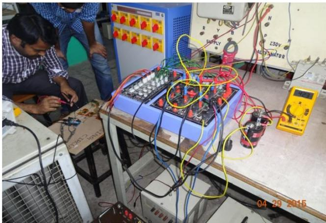
Unified power Flow Controller (UPFC) Test Bench
