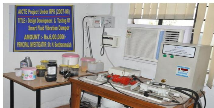
**Smart Fluid Vibration Damper set up of MED**
