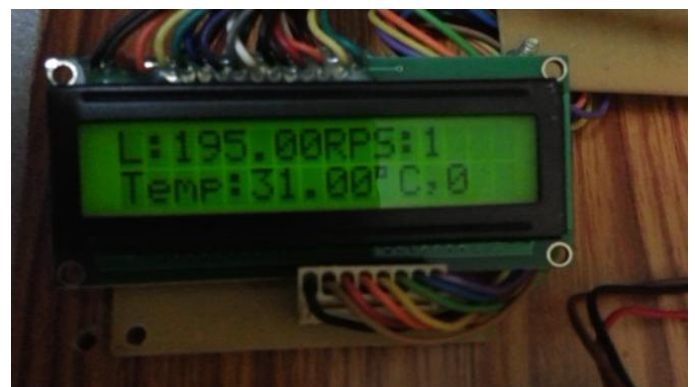
Fig 3 LCD Display showing Level,RPS & Temperature
