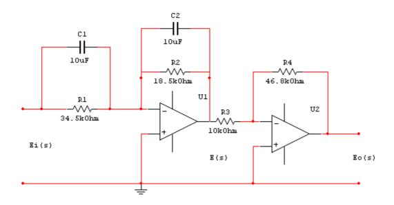
The closed loop transfer function equation for the compensated system becomes
