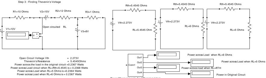
Power Measurements for different resistors
