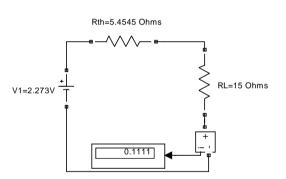
With all the sources in the network Current through Load Resistor 15 Ohms : I=0.1111A
