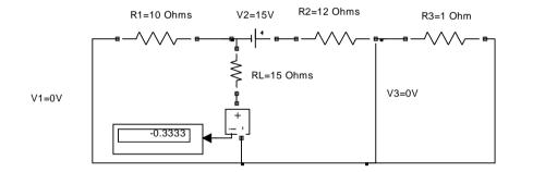
Current through Load Resistor 15 Ohms :
