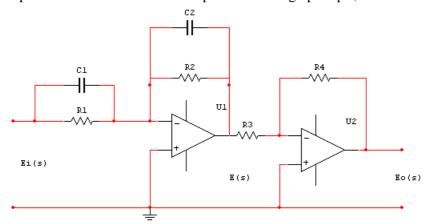
$$\frac{Eo(s)}{Ei(s)} = \frac{R_2}{R_1} \frac{R_4}{R_3} \frac{R_1C_1s+1}{R_2C_2s+1} = \frac{R_4C_1s+\frac{1}{R_1C_1}}{R_2C_2s+\frac{1}{R_2C_2}} = K_c \alpha \frac{Ts+1}{\alpha Ts+1}$$
