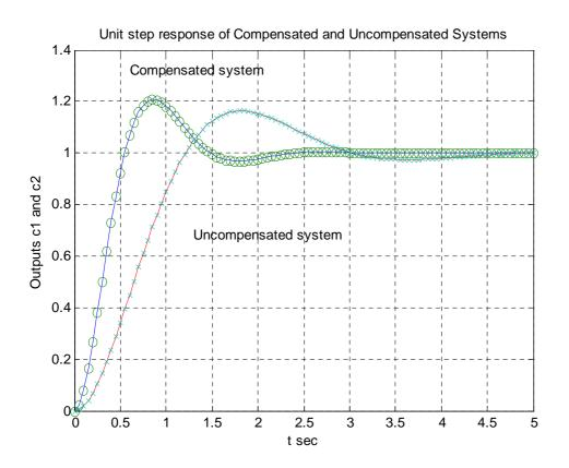
For Lag Compensator The closed loop transfer function equation for the compensated system becomes
