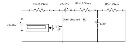
Open Circuit Voltage Vth = 2.273V Thevenin's Resistance = 5.4545Ohms Current through Load Resistor 15 Ohms IL = 0.1111A R1=10 Ohms V2=0V R2=12 Ohms R3=1 Ohm
