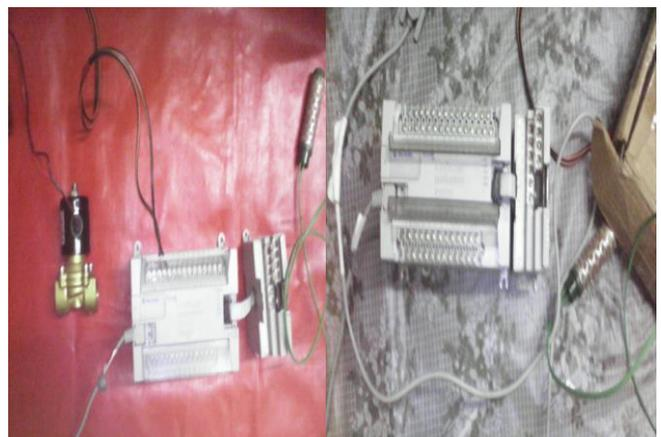
**Drip Irrigation using PLC setup**
