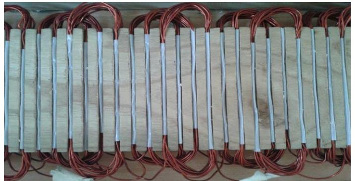
The arrangement of the winding for MAGLEV Train
