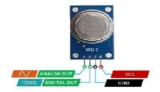
Aim:- To interface Arduino with MQ2 gas sensor module
