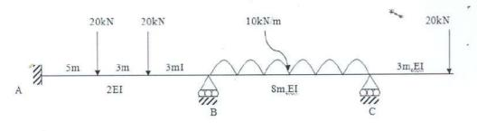
8. Analyze the given continuous beam by moment distribution method. Also draw BMD and SFD. If Sinking @ B = 75/EI and Sinking @ C = 25/EI. (CO2)
