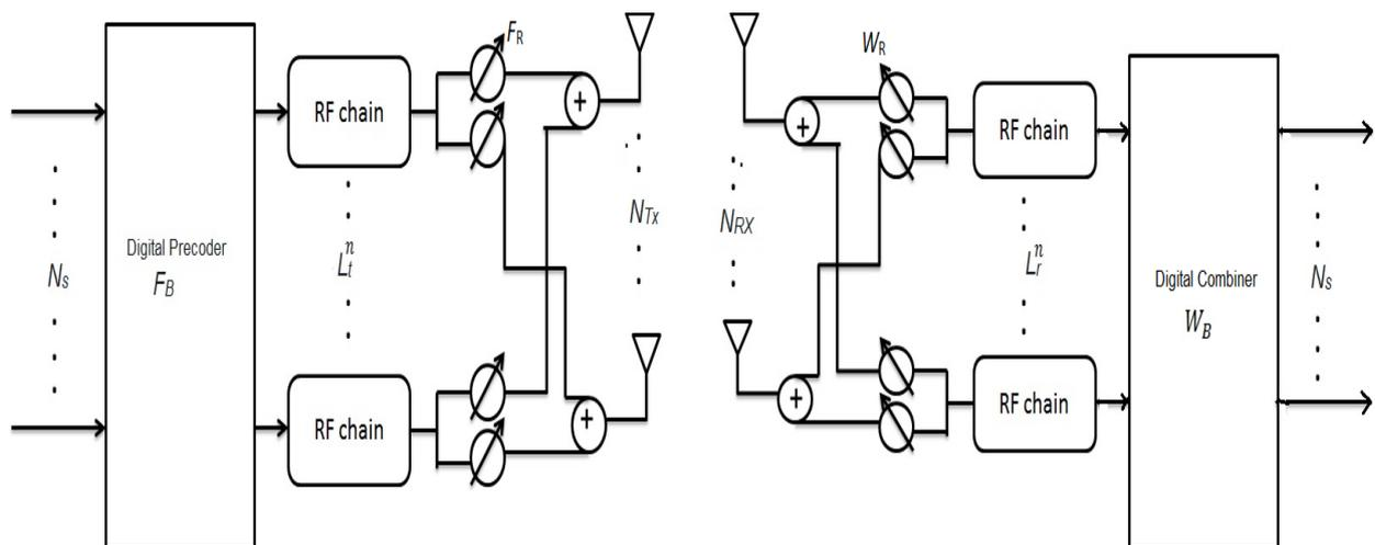
**Figure 1:** A HPC fully connected structure in mm-Wave MIMO system
