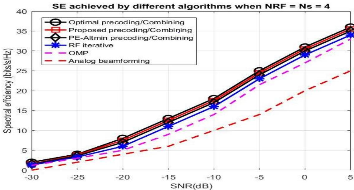
**Figure 3:** SE vs SNR for different algorithms for  $N_{T_x} = 144$ ,  $N_{R_x} = 36$
