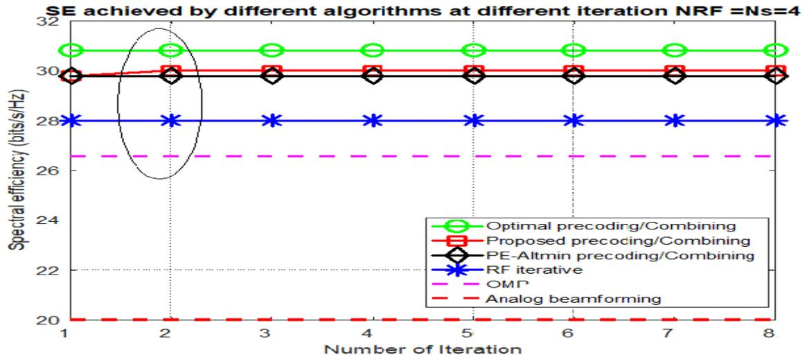
Figure 4: SE vs no. of iteration by different algorithms (Lt=Lr=NRF=Ns=4) and SNR=0dB
