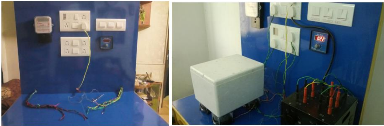
Fig.1 Experimental set-up with (a) Electrical circuit connections (b) transformer, modules, heat-sink and container connections
